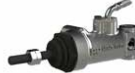
CP6467, PULL TYPE, TRUNNION MOUNTED, FOR ABS & HIGH PRESSURE INLET = SPECIAL PLUG-IN, OUTLET = M10X1.0 M8X1.25 PUSH ROD
