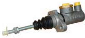
CP4623 PUSH TYPE SHORT STROKE FLANGE MOUNT OFFSET INLET = 7/16UNF, OUTLET = 3/8UNF * 5/16UNF ROD - 115MM(PRT115) / 160MM(PRT160) * M8X1.25 ROD - 115MM(PRM115) / 160MM(PRM160)
