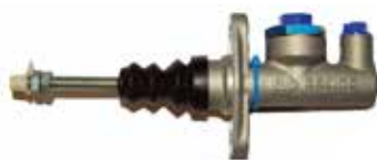
CP2623 PUSH TYPE SHORT STROKE FLANGE MOUNT INLET = 7/16UNF, OUTLET = 3/8UNF * 5/16UNF PUSH ROD - 115MM(PRT115) / 160MM(PRT160) * M8X1.25 PUSH ROD - 115MM(PRM115) / 160MM(PRM160)
