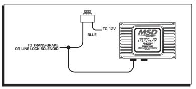
Figure 3 Wiring the 2-Step Rev Limit.
