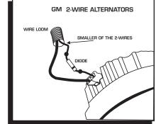
Figure 7 Installing the Diode to a 1973-1983 GM Vehicle.
