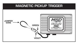
Figure 10 Checking for Spark with the Mag Pickup.
