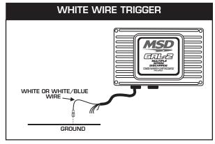
Figure 9 Checking for Spark with the White Wire.
