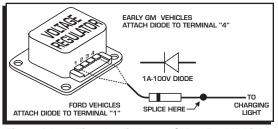
Figure 6 Installing the diode to a GM or Ford Vehicle.
