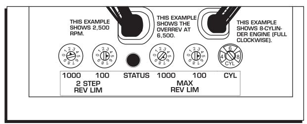
Figure 2 Rev Limiter sample setting.
