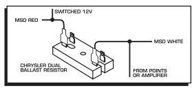
Figure 5 Wiring the Dual Ballast Resistor.
