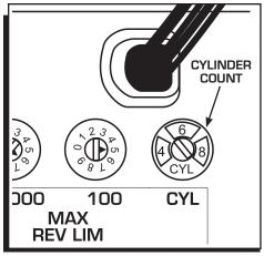
Figure 1 Programming the Number of Cylinders.
