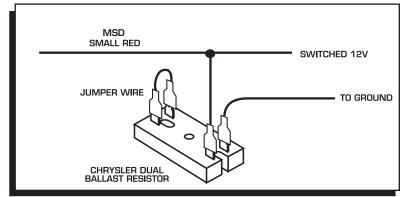
Figure 8 Wiring the Dual Ballast Resistor for Run-On.
