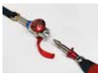
8111-K RACING NET Racing Net (generally used for door positions, ease of driver changes), Push-Button Release, Kevlar Webbing, Meets FIA 8863/2013. Only made in black, available for left side of driver or right side of driver.
